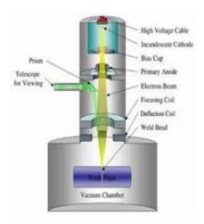
The Material used in EBM is metal powder that melts and forms a 3D part layer by layer by means of a computer that controls electron beam in high vacuum. Contrary to SLS, EBM goes for full melting of the metal powder. The process is usually conducted under high temperature up to 1000 °C.
